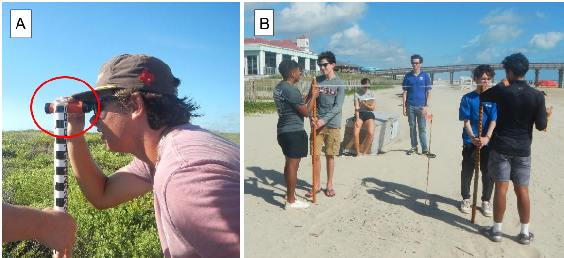
Figure 2. Students use (A) a sighting level to determine vertical offset between Emery rods and (B) a metric tape to measure horizontal distance.
