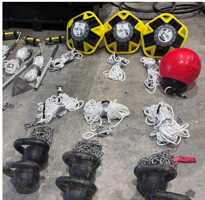
Figure 10 Schematic of Spotter wave buoy deployment setup (left) and pre-deployment instrument mounting setup (right) for Spotter wave buoys (yellow) with rope lines, anchors, and floater buoys (red).
