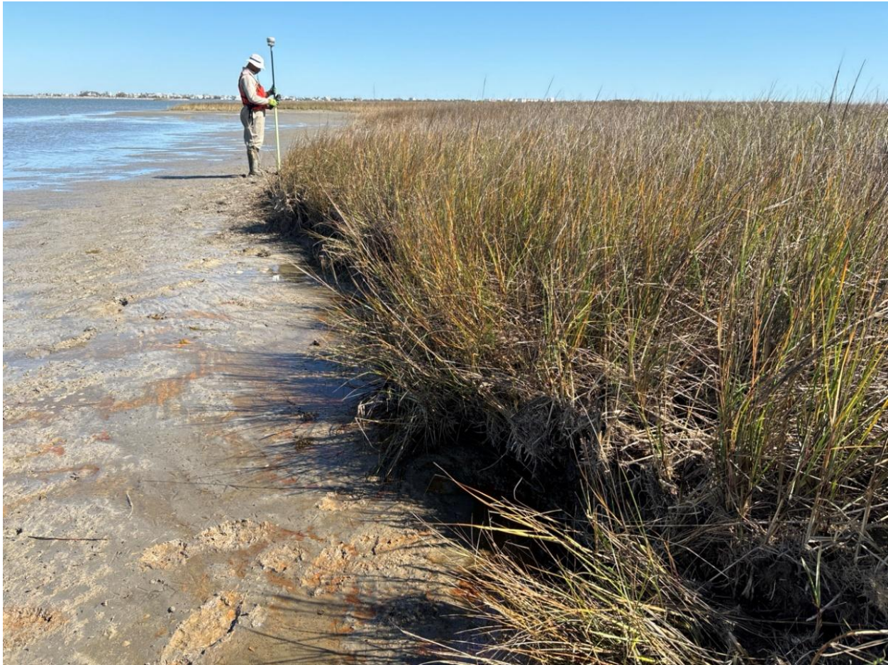
Figure 7. Topographic survey of marsh edge position.
