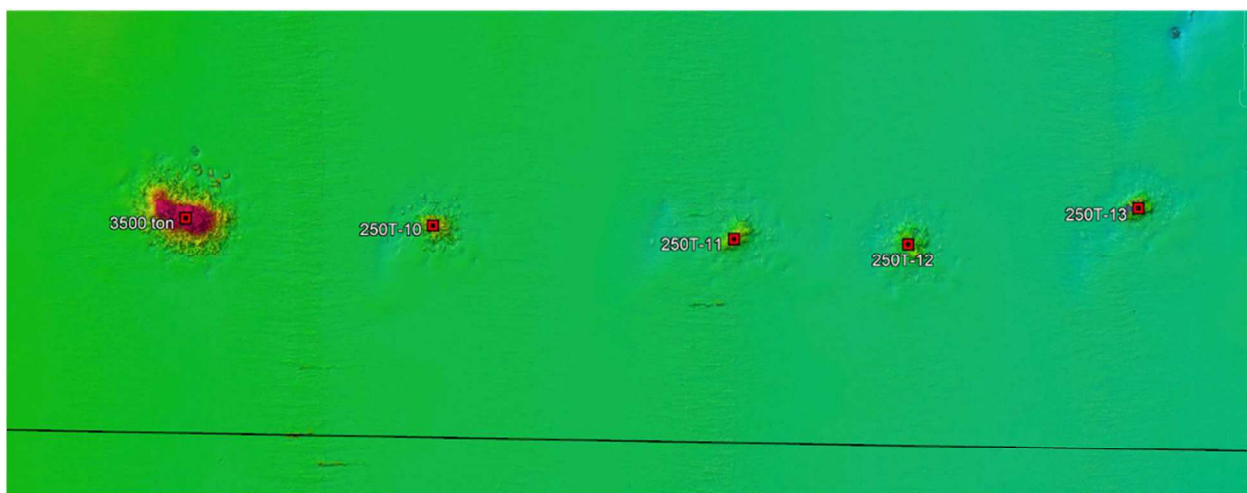
Figure 8. Overview of the 250-ton railroad tie patches (10-13) and the 3500-ton pile at the Rio Grande Valley Reef (PS-1105). Image was generated from 400 kHz multibeam recordings in August 2025.
