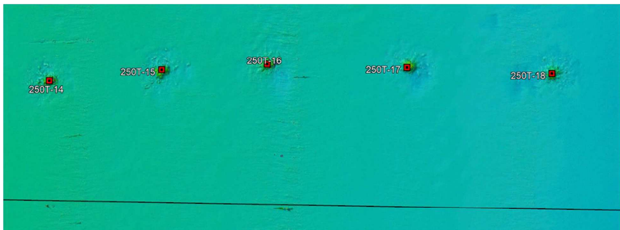
Figure 9. Overview of the 250-ton railroad tie patches (14-18) at the Rio Grande Valley Reef (PS-1105). Image was generated from 400 kHz multibeam recordings in August 2025.
