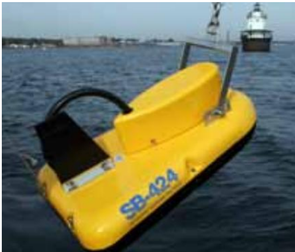
Figure 3-8: An Edgetech SB424 subbottom profiler was used during this survey.
