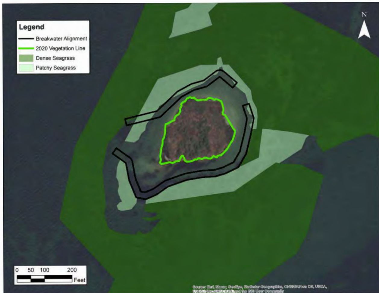
Figure 16. Plan view of Alternative 1: riprap breakwater
