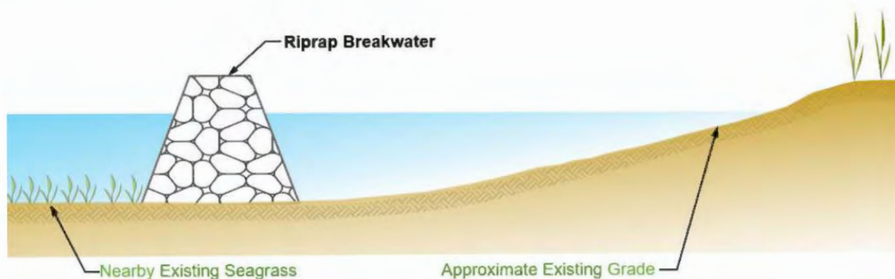
Figure 16. Plan view of Alternative 1: riprap breakwater
