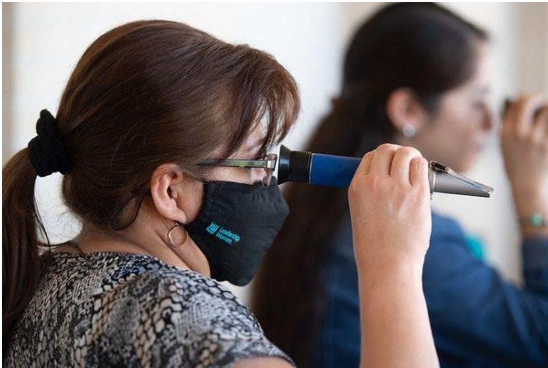
Figure 7. Measuring the salinity of bay water samples using refractometers.
