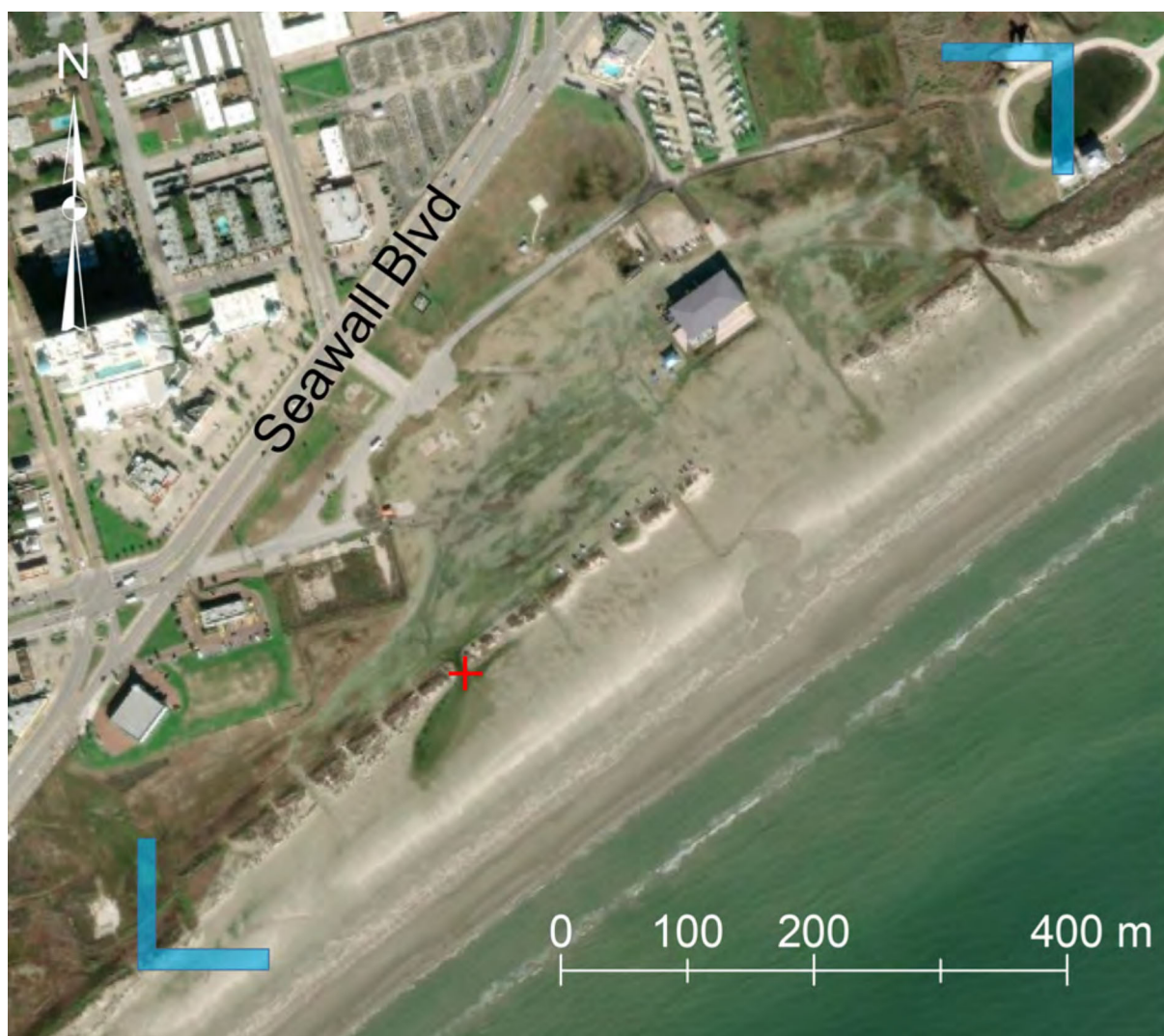
Figure 5. Zoomed in satellite image of Stewart Beach (Eastern Beach study site). The corner brackets (L) mark the north-east and south-west boundaries (Table 1) of the target unmanned aerial vehicle (UAV) survey area. Sediment samples were collected at the location marked by a cross (+).
