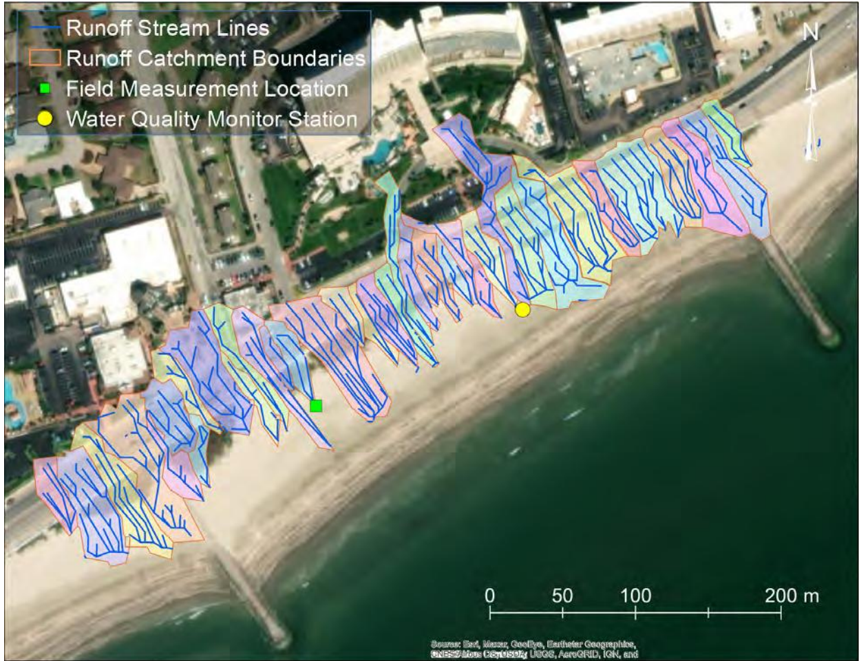
Figure 8. Runoff catchments and surface stream network calculated for the CB site (53 rd Street Beach).
