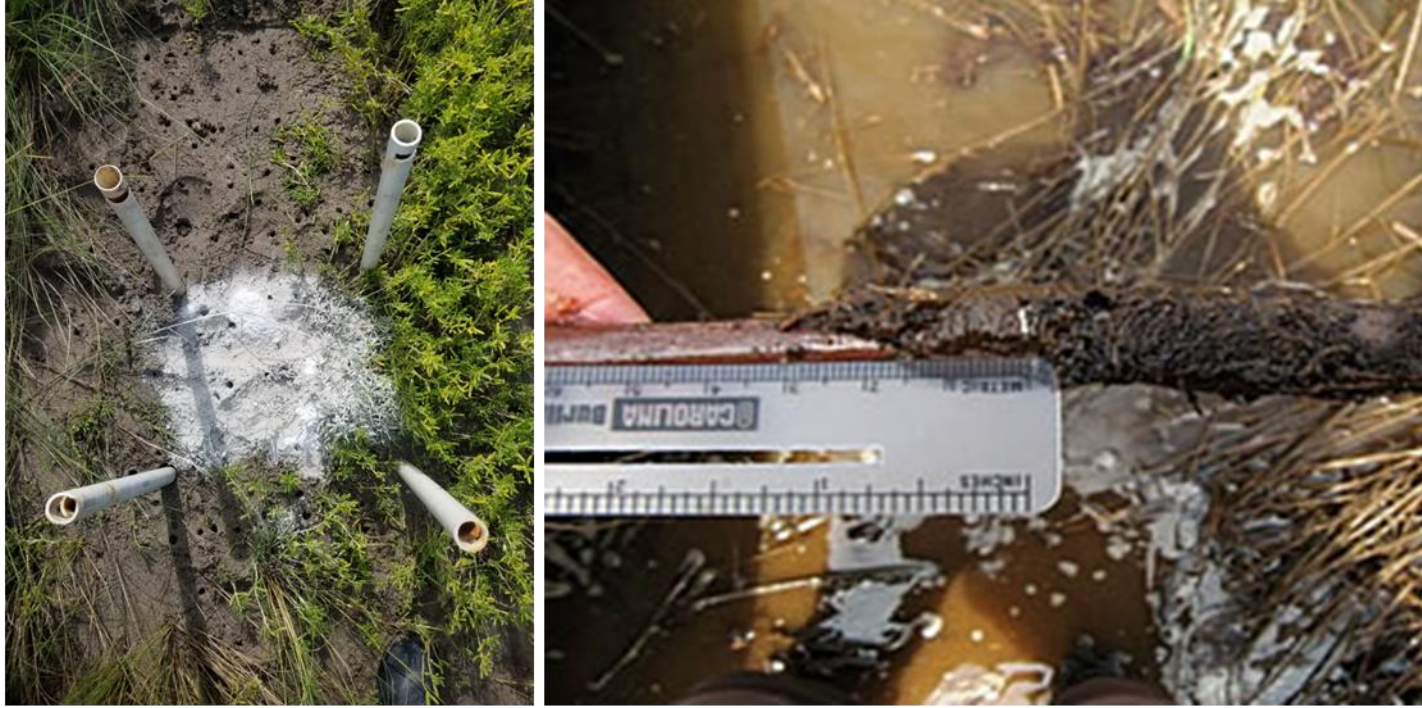
Figure 4a. (left) Feldspar set on the wetland surface as a marker horizon (PINS site). b. (right) a core showing s above the marker horizon (from: https://www.tidalmarshmonitoring.net/monitoring-methods-marker-horizons ).
